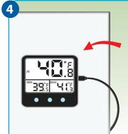
Attach the digital display to the outside of the refrigerator, either on the door or on the side.
