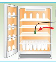
Place the probe in the center of the refrigerator.
